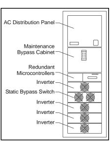
critical load, the system will automatically transfer to the static transfer switch and disconnect from the DC source. The static transfer switch (standard) will make a seamlessly, uninterrupted transfer from the critical load to an alternate AC power source where the inverter power was synchronized to (utility power or another protected AC source). The availability of the Alphatran N+1 on-line mode with a backup source present is greater than 99.9999%.
