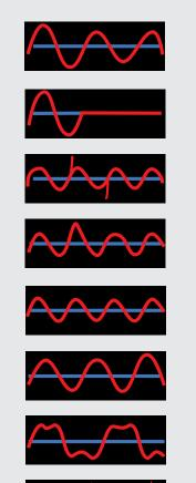
SAGS a sudden decrease of input voltage for a short time. BROWNOUTS are steady decrease of input voltage for a long time. The load is still supplied but at a voltage below its tolerances.
